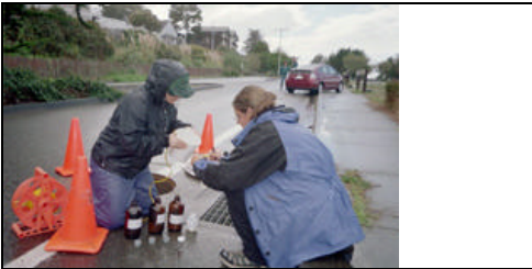
Composite samples were collected from the manhole sites with a bucket.
