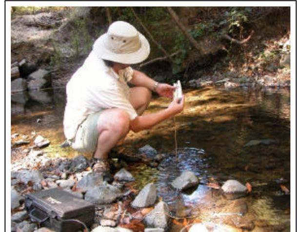
**Citizen Monitor Tom Austin takes readings for pH and Electrical Conductivity using handheld meters on a stretch of Dutch Bill Creek .**
